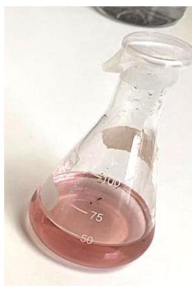
Fig. 2 Vitreous biomaterial sample solubilized in water for 24 hours with constant agitation, the characteristic purple color of the anthocyanins of the red polyphenols can be observed.
