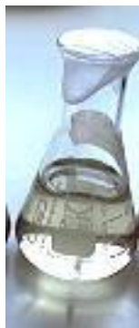
Fig. 4. Sample treated for 24 hours at constant temperature and agitation with acetone. It is possible to be seen in contrast with figure 1 the slight yellow tone of the sample product of the solubilized lipids.
