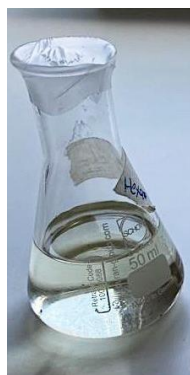
Fig. 5. Sample treated for 24 hours with hexane at constant temperature and agitation. In contrast to Figure 1, the faint yellow coloration of the sample is seen, probably the product of the extraction or only the location of waxes and fats.
