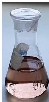
Fig. 3. Sample treated for 24 hours at constant temperature and agitation with ethanol. The red or purple color of the solvent shows the release of different polyphenols.
